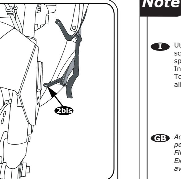
**GB** Fasten Termoscud® on both sides, using the scooter original's fasteners\*, threading them through the holes at the end of the straps 2bis.
