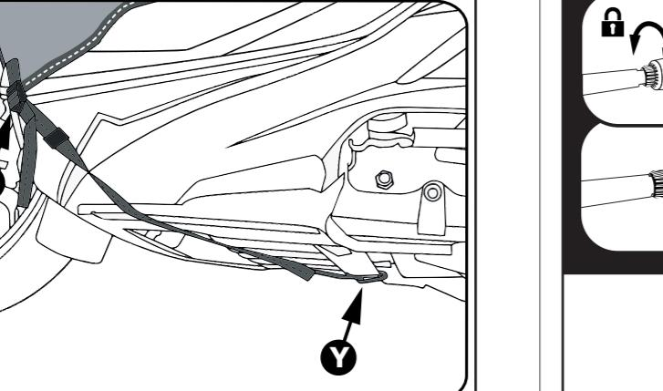
**GB** Fasten the hook of the extension strap Y to the edge of the bodywork under the footboard. Close the buckle and tighten the straps 2.
